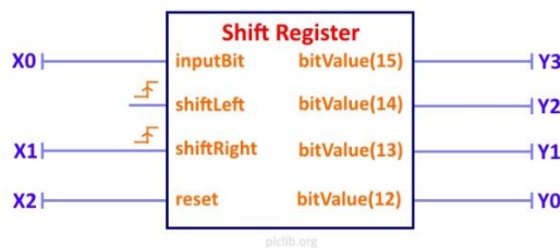
Figure 30. A block diagram representation of the shift register, plus its inputs and outputs.
