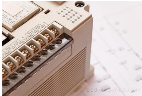
Figure 5. A typical Programmable Logic Controller (PLC). Image © istockphoto.com/Igor Mazej.
