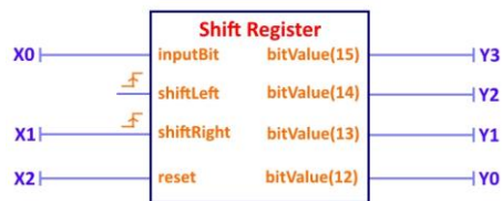
Figure 35. A function block representation of the shift register.
