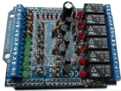
Figure 6. The Velleman Input/Output Shield offers a useful range of pre-configured inputs and outputs.
